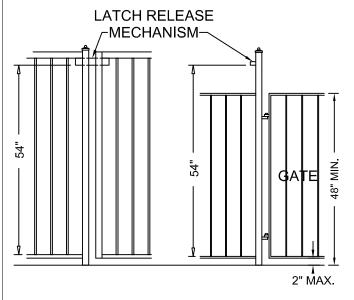
LATCH RELEASE MECHANISM LOCATED AT 54" OR HIGHER FROM THE BOTTOM OF THE GATE.
