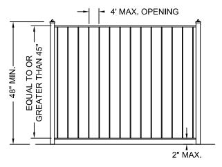
IF HORIZONTAL MEMBERS ARE EQUAL TO OR GREATER THAN 45" APART VERTICAL SPACING SHALL NOT EXCEED 4".
