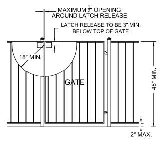
LATCH RELEASE MECHANISM LOCATED LESS THAN 54" FROM THE BOTTOM OF THE GATE.
