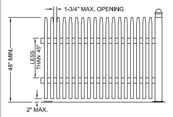
IF HORIZONTAL MEMBERS ARE LESS THAN 45" APART, VERTICAL SPACING SHALL NOT EXCEED 1-3/4" INCLUDING CYCLONE FENCES.
