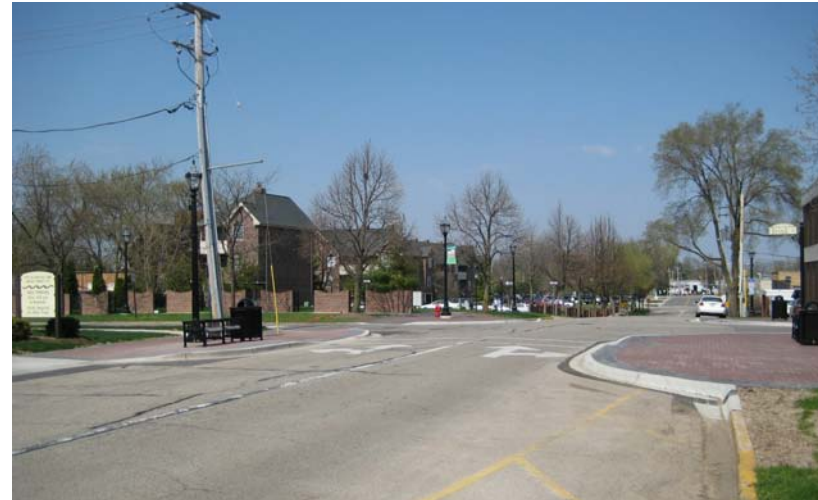
Figure 4.13. Examples of curb extensions
