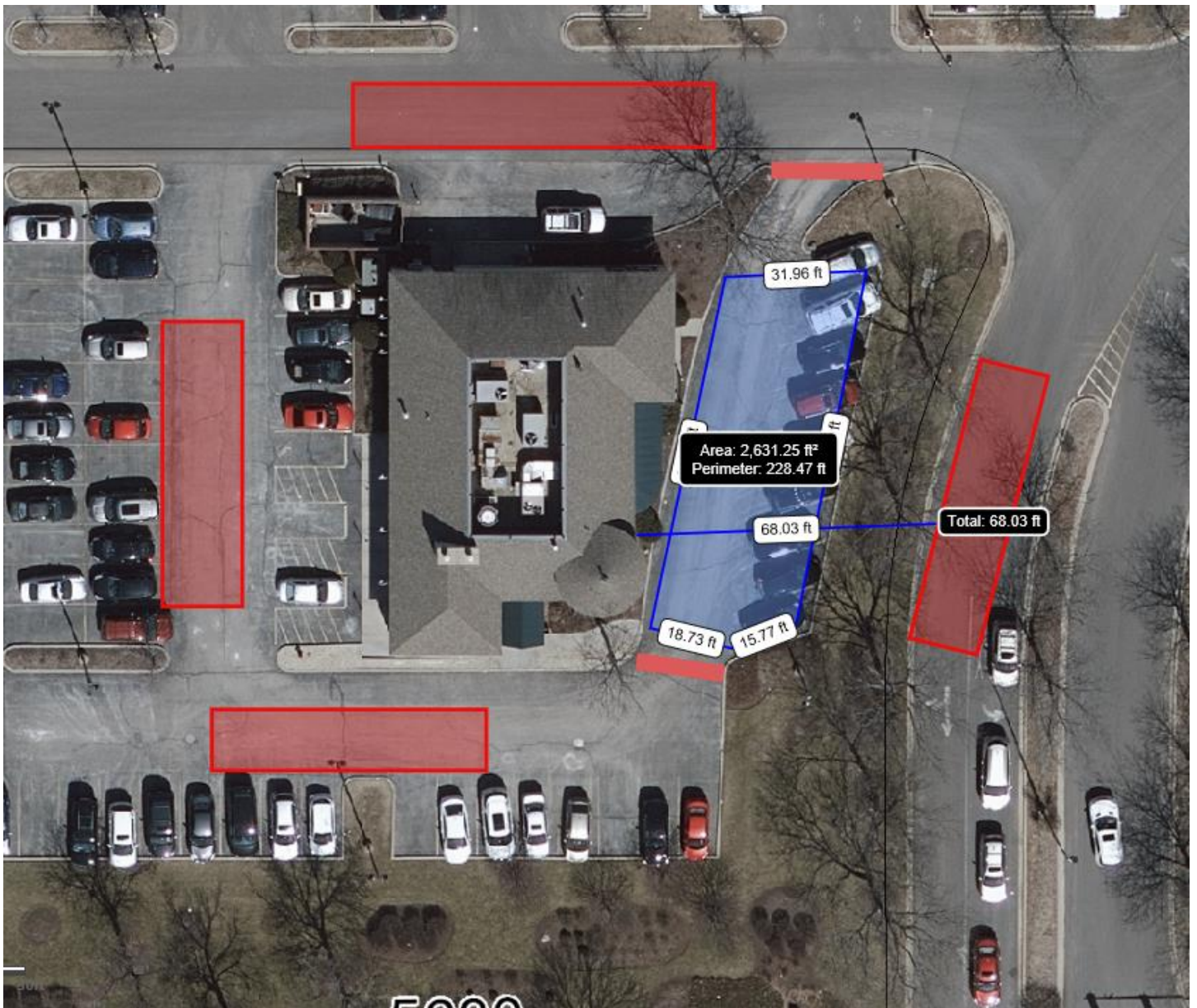
Fire Truck access around the building
