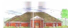
Mansard roofs should be appropriately scaled so as not to dominate the elevation.
