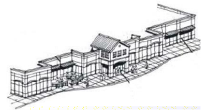
Various details recommended to be used to create shadow patterns and depth on wall surfaces.
