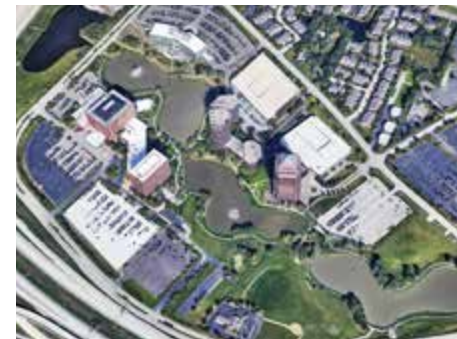
Example images of stormwater detention facilities serve a dual-purpose of mitigating stormwater runoff and as a central open space where buildings and activities orient toward to.
