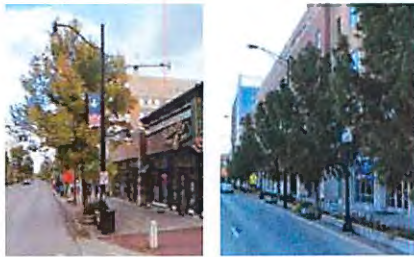
Examples of dual-scale lighting fixtures. Alternating pedestrian- and auto-scale fixtures can be an appropriate alternative.
