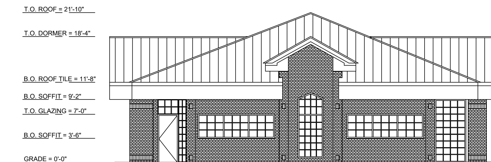
1 EAST ELEVATION SCALE: 1/4" = 1'-0"
