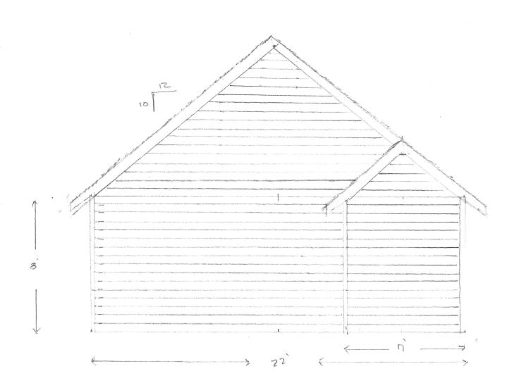
ZX8 ceiling joist IXS TIC 2×10 Ridge Board 1 x 8 Facine The Klyn soft it 1/2 ply roof sharing 242 / 1/2 ply interven for window/ soor thates compe door header 11 1/8 LUC (2 math)
