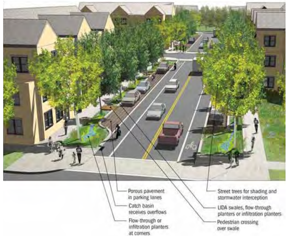
Figure 60. Greener Streetscape using LID practices. Source: "Greening the Code" Washington County, OR.
