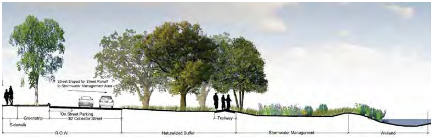
Figure 57. Stormwater Treatment Train within Conservation Development.
