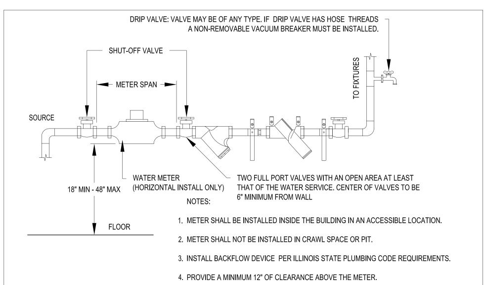
5. METER TO MEET MANUFACTURERS SPECIFICATIONS FOR UPSTREAM PIPE REQUIREMENTS.
