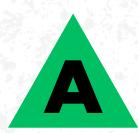
Class A Extinguishers will put out fires in ordinary combustibles, such as wood and paper. The numerical rating for this class of fire extinguisher refers to the amount of water the fire extinguisher holds and the amount of fire it will extinguish.
