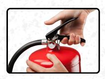
**SQUEEZE** the lever above the handle: This discharges the extinguishing agent. To stop the discharge, release the lever.
