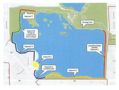
The path will be eight-foot wide gravel with one-foot shoulders. Construction will be completed in phases. Segment 3, located near the southwest corner of the lake was completed in 2024. Bids
