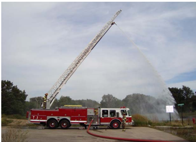
Truck 381 and crew conducting a master stream drill.
