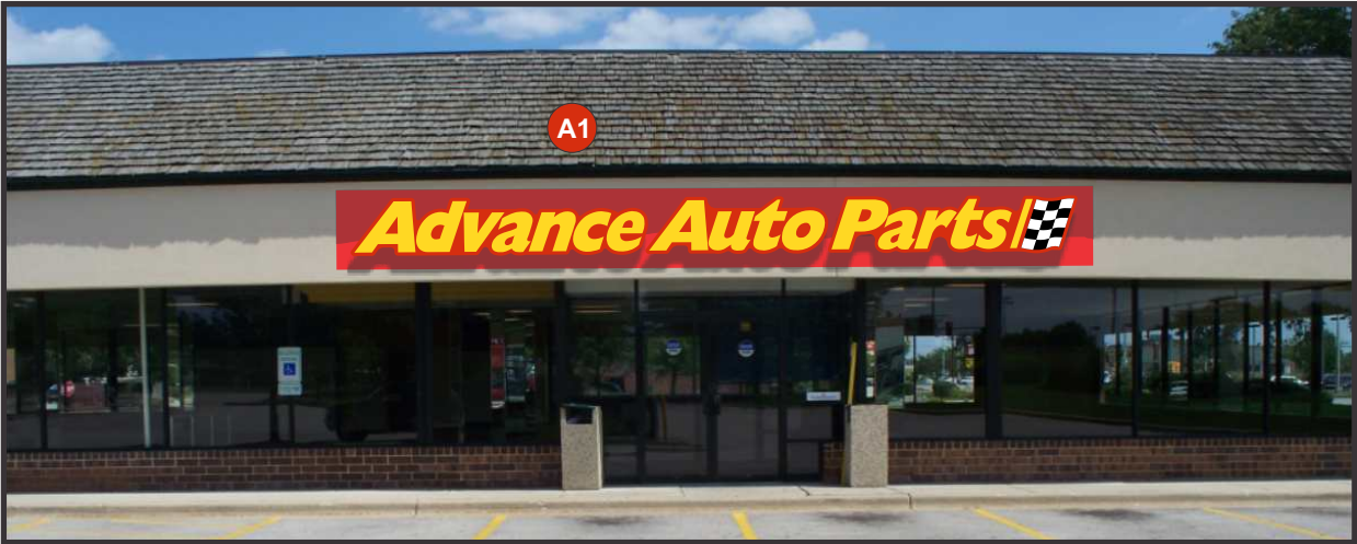
Proposed West Elevation - 3'-6" x 33'-4" Area Behind Sign Painted Red, Rest of Facade Color to Remain As-Is
