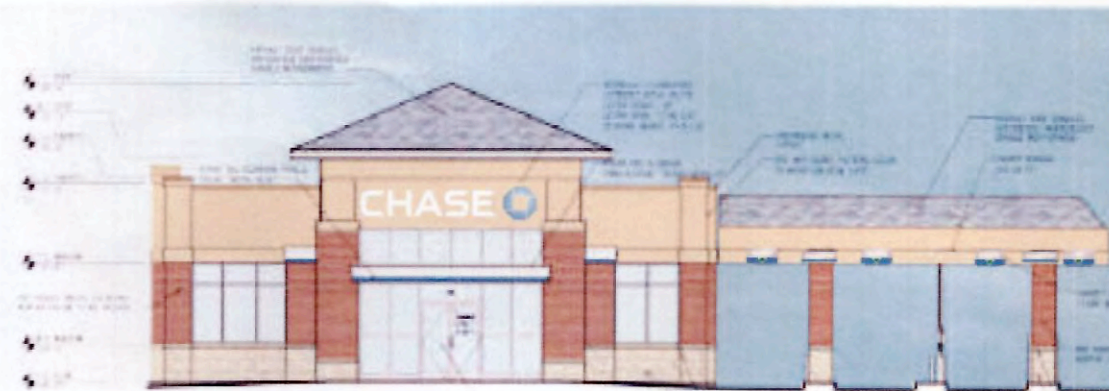
WEST ELEVATION - (WHITE LTRS / BLUE OCTAGON) - LIF-WBO-30 Scale: 1/16" = 1'-0"
