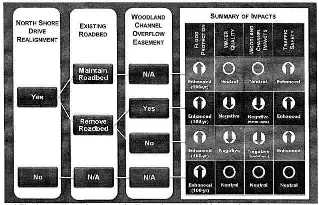
\* Flood protection enhancement is due to the separate culvert and channel improvement, which is recommended with or without the North Shore Drive realignment.
