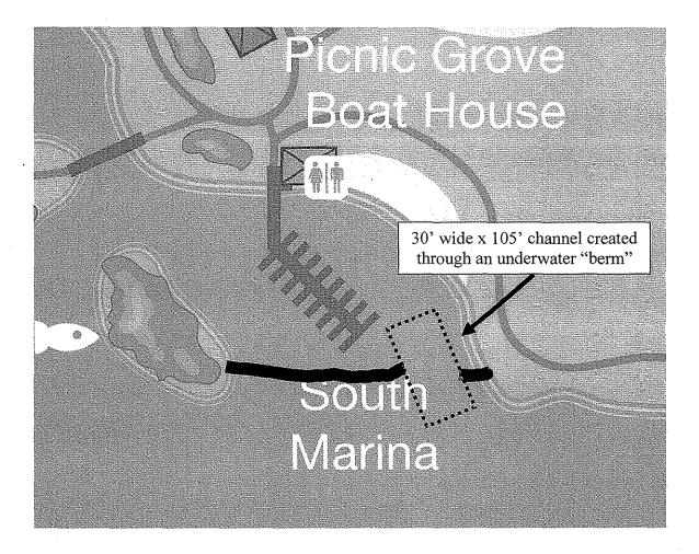
The area and size of the channel was designed so that it could be constructed by an earthwork excavator working close to the shore. This keeps the cost of construction lower than using other alternative dredging methods (i.e. using a barge). The specifications require that the contractor remove approximately 687 cubic yards of materials and move these materials closer to the shore of the lake, or further out into the lake.
