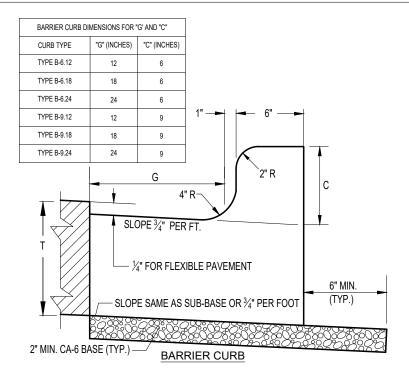
CONTRACTION JOINTS AND EXPANSION JOINTS SHALL BE INSTALLED IN THE CURB OR CURB AND GUTTER IN PROLONGATION WITH JOINTS IN ADJACENT P.C.C. PAVEMENT OR BASE COURSE.
