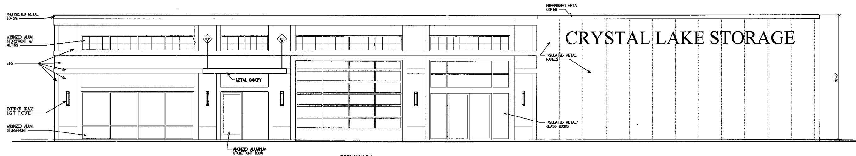
PRELIMINARY BUILDING 'A' West Elevation SCALE: 1/4"=1'-0"
